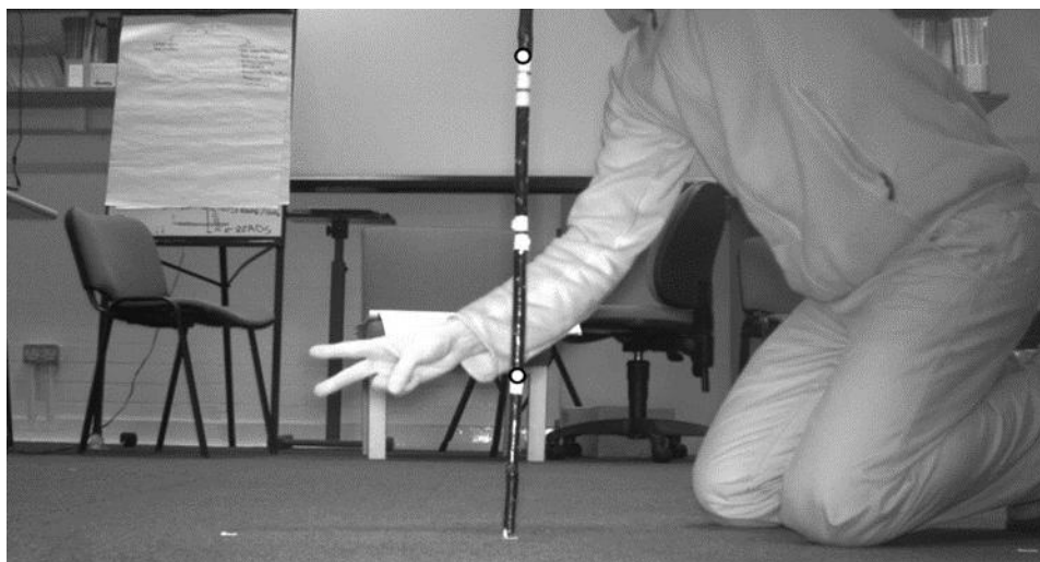
Figure A6. A camera calibration image with pole in position 2 m from the camera.
